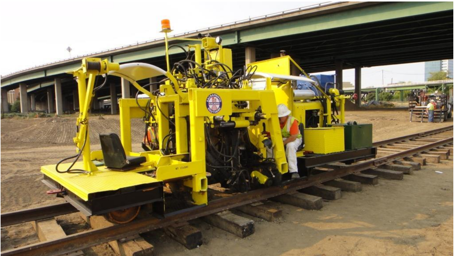
Bring in the Super "B": Mike H. pilots the spiker onto the new track to begin driving spikes into these hard oak ties
